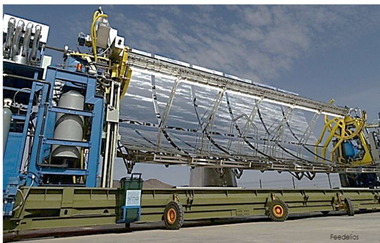
The industrial-sized solar microwave oven (SMO) for valorization of organic biomass and organic waste
