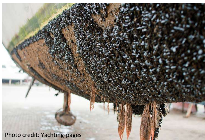
Yacht hull showing extensive marine fouling.
