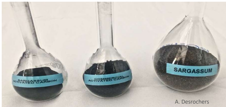
Activated carbon made with sargassum displayed alongside a commercial sample of activated carbon (centre)
